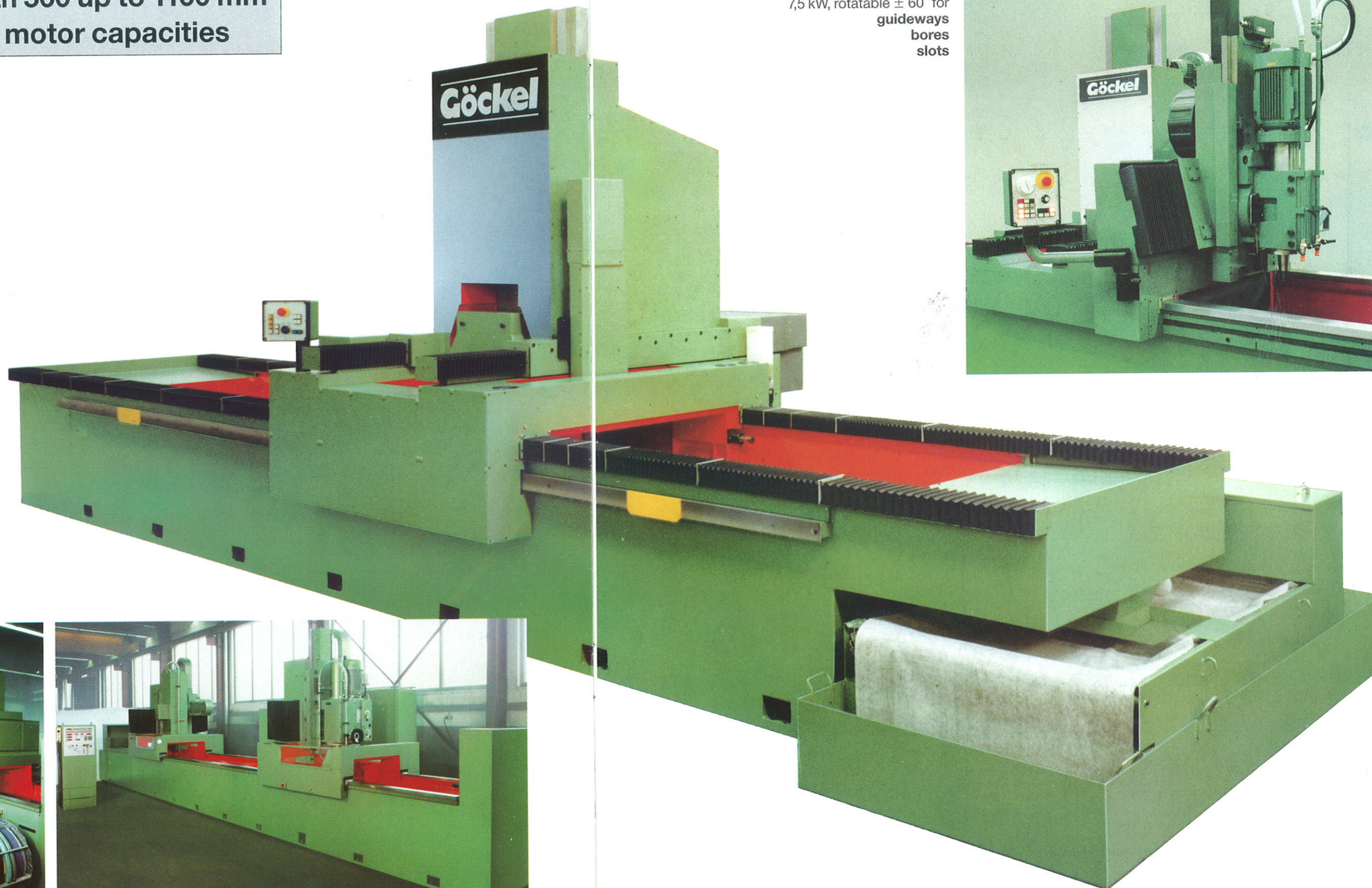
6 Combined production machine with milling and grinding carriage. CNC controlled, 6 axes
